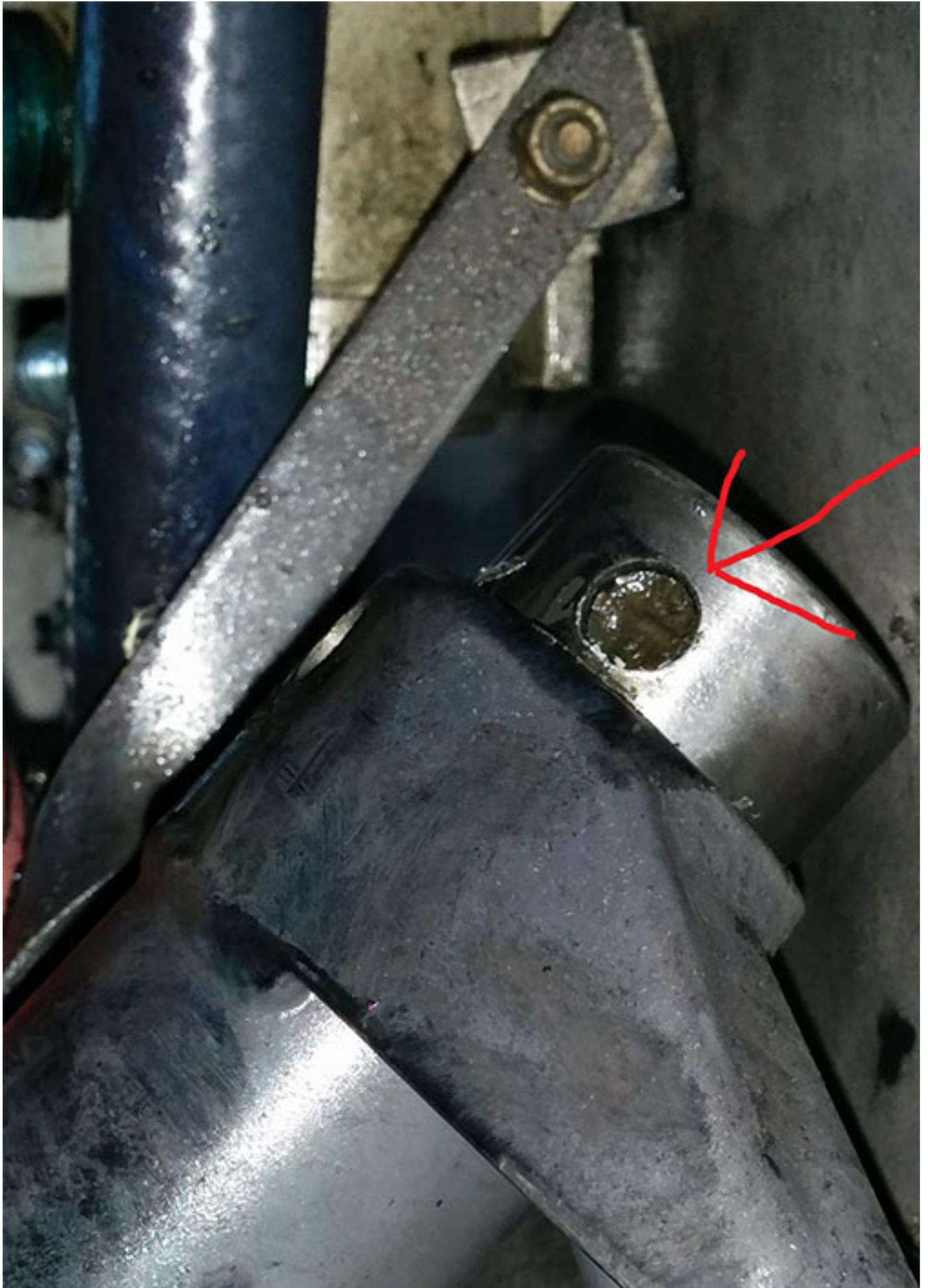
**We highly recommend performing Van's new Service Bulletin to check the stop collar orientation before further flight:**
