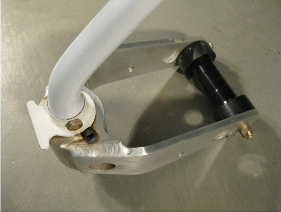
Sheared leg retainer bolt from incorrectly installed stop collar:
